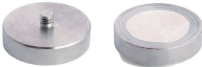
CMCP-MB019 Large Magnetic Base for flat surfaces, 110 Lbs Pull Strength, 1.60" diameter, 0.4" Height, ¼"-28 Stud
