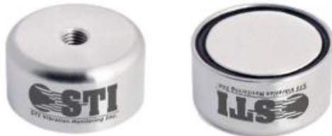
CMCP-MB02F Medium Magnetic Base for flat surfaces, 30 Lbs Pull Strength, 1.00" diameter, 0.6" Height, ¼"-28 Threaded Hole
