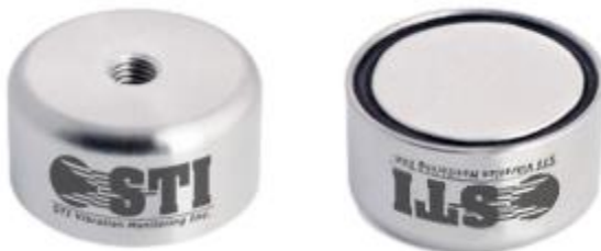
CMCP-MB03F Medium-Large Magnetic Base for flat surfaces, 55 Lbs Pull Strength, 1.20" diameter, 0.6" Height, ¼"-28 Threaded Hole
