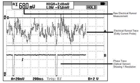
Screenshot from Fluke ScopeMeter above Shows 0.3 mils of Electrical Runout
